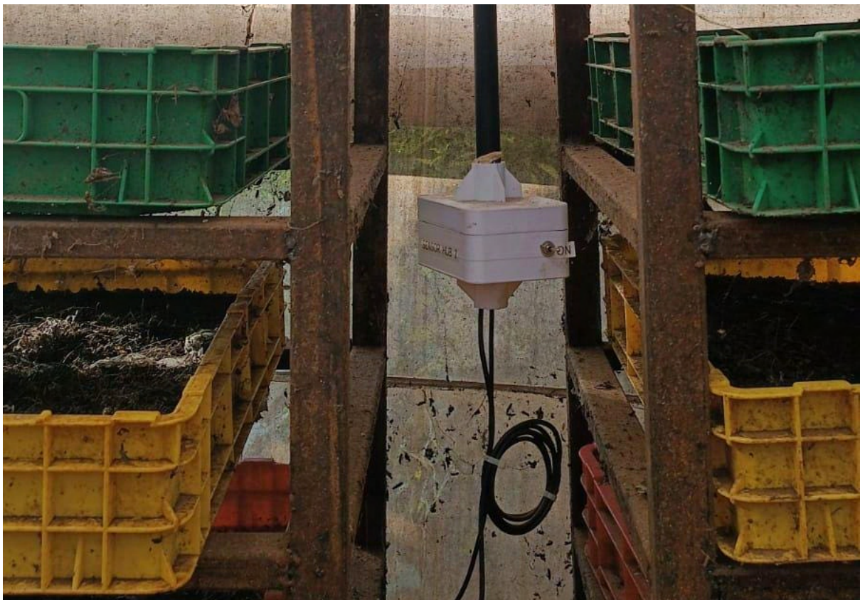
PHOTO CREDIT: ZIHANGA LTD Sensors deployed at Zihanga Ltd, to monitor optimal conditions for BSF production..
