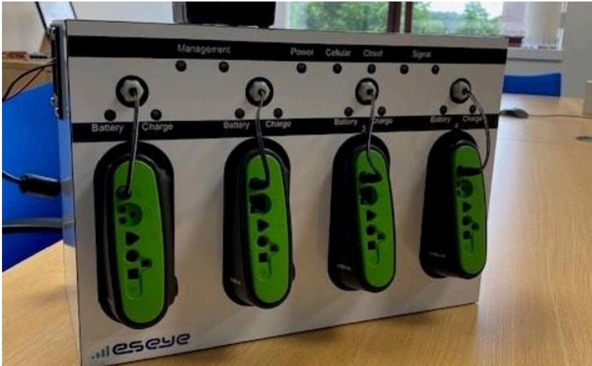
A prototype battery charging station developed throughout the pilot for charging four lithium-ion batteries.
